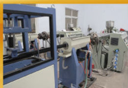
Pipe Production Line
